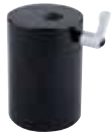
Counter Weight P/N: QC2SCM2700 May be attached to opposite side of gear rack when off balance loading of equipment is encountered such as when running two torches on one side. Standard operation does not require counterweights.
